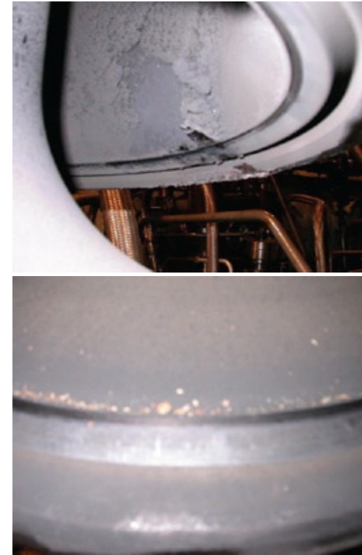
Figure 10: Photographs of the valve spindle and seat ring surfaces after 1,000 hours [6].
