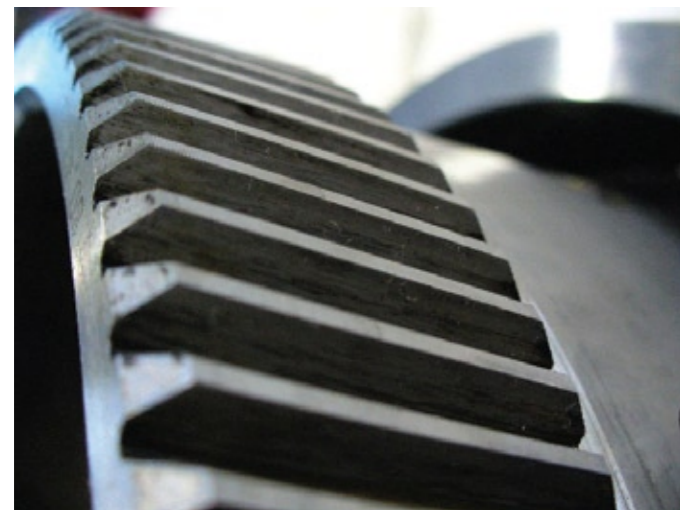
Figure 17: Photograph of the inner helix gear after 31,882 hours.
