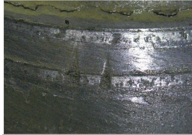
Figure 5: Valve spindle with extensive dentmarks and beginning of blow-byes (W-type geometry of bottom piece).
