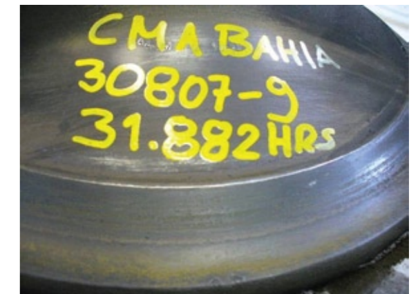
Figure 13: Photograph of valve spindle seat surfaces after 31,882 hours.
