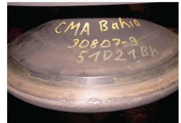
Figure 14: Photograph of valve spindle seat surfaces after 37,505 hours.
