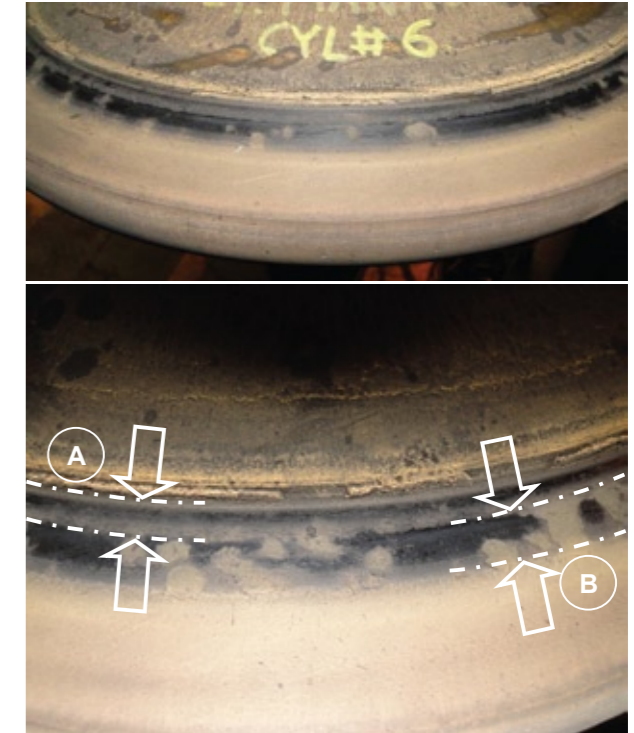
Figure 20: Valve spindle seat with removed glassy-deposits (chamber type geometry of bottom piece with modified seat angle for higher seating pressure).
