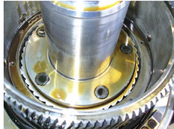
Figure 15: Photograph of the rotator gear and free-wheel after 31,882 hours.
