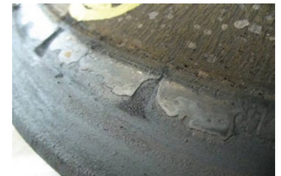
Figure 4: Valve spindle with extensive "glassy-deposits" and beginning of blow-by.
