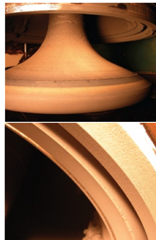
Figure 11: Photographs of the valve spindle and seat ring surfaces after 9,100 hours [6].
